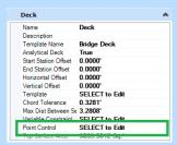
In the point control dialog, the user can control the different points of the deck with elements created in ORD or using the civil tools in OBM. The points can be control horizontally, vertically, or both. To add a point control, select the direction from the drop-down menu, then click the Select button to identify the plan element in the screen. Once identified the plan element name will appear in the Path column.
