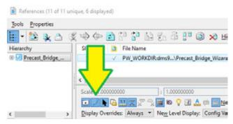
If Accu-draw is not already active, turn it on by pressing F11 on your keyboard or navigating to Home > Primary and selecting Toggle Accu-draw to turn on XY coordinatebased drafting tools. You can dock the XY input boxes to the bottom of your window.
