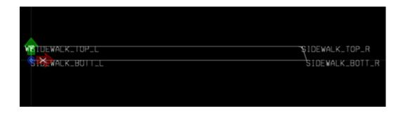
7. Adjust the point constraints to attach the sidewalk bottom to the bridge deck, add a 34" chamfer to the left top and left bottom corners of the sidewalk, and add a 2" fillet to the top right corner to represent the curb per TxDOT standard drawing BRSM. See Sidewalk\_Top\_R Point Constraints on how to adjust your toe offset.
