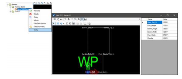
20. The template is meant to be used as the left side of a bridge, to create the right side right click on the template name and select Copy, then select the newly copied template, right click on it and select *Mirror* and rename the template so that it indicates is the right side.
