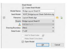
The section drawing will get referenced into the sheet selected, in this case Bridge Layout Sheet 01.
