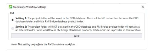
Unlike LEAP, the user can select exactly what components to transfer to RM, and the user can select all units, and all bridges, RM will always export the active Bridge/Unit.
