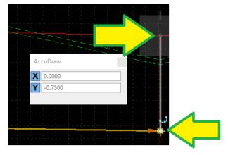
Once the line below the abutment cap is in place, we will draw the lines along the wingwalls using the previously created line as our start point and ending at 1 foot before the end of the wingwall at the top.
