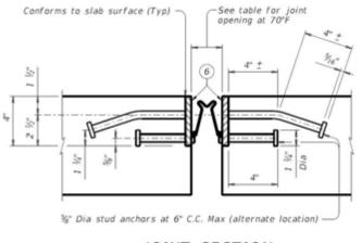
JOINT SECTION Showing R J Watson strip seal. Other strip seals are similar.
