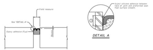
Figure 3-7: Example of pre-formed compression seal.
