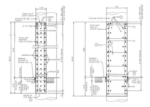
Figure 7-3. Sections showing single-sided and double-sided deflection walls.
