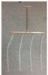
Figure 2-2. A chain drag made from copper tubing and steel chain.
