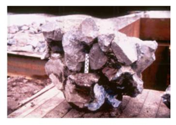
Figure 13-3: Grouted Stone Protection – Conglomerates
