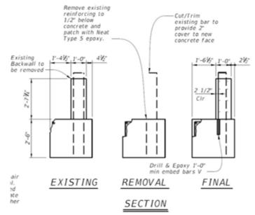
Figure 3-15: Example of backwall reconstruction.
