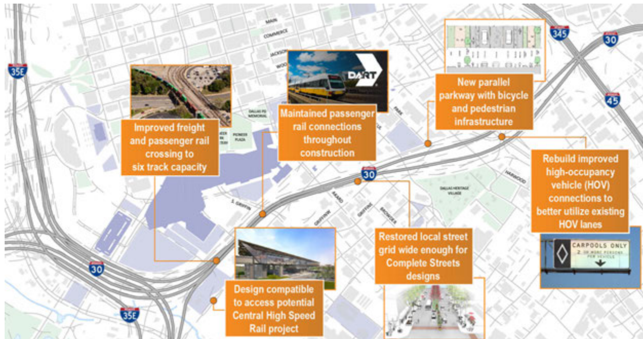
Figure 11 Multimodal Improvements in the I-30 Canyon Project
