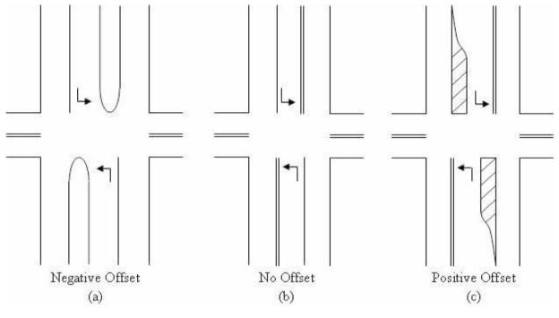
Figure 5-1 Left-Turn Lane Offset Source: FHWA-HRT-09-035
