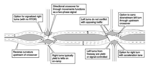
Figure 6-4 Example of a DDI intersection and its key characteristics Source: FHWA-SA-14-067
