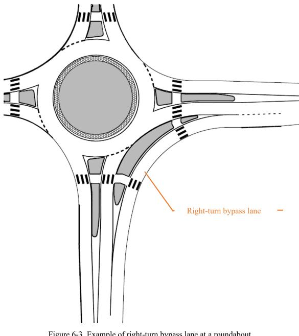
Figure 6-3 Example of right-turn bypass lane at a roundabout Source: NCHRP Report 672
