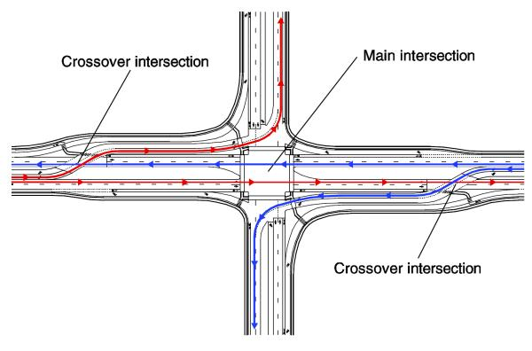
Figure 6-5 Example of a DLT intersection design sketch Source: FHWA-SA-14-068
