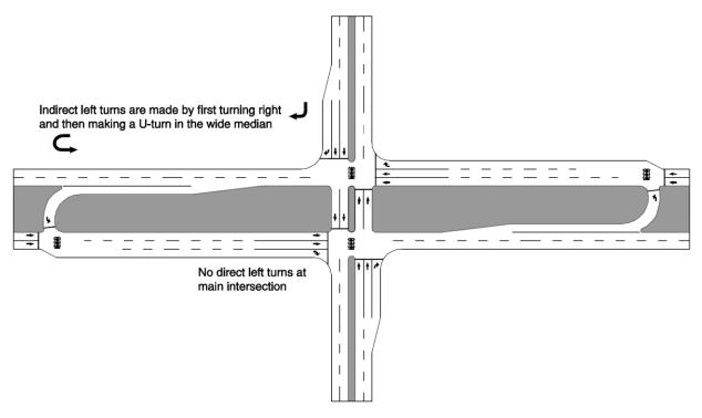
Figure 6-6 Example of a MUT intersection Source: FHWA-SA-14-069
